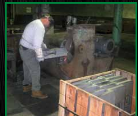
Workers grind off rough edges and give casting a finish of paint, if requested.
