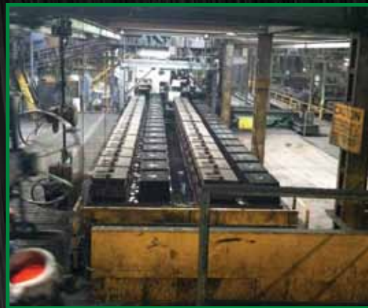
Molds are indexed to shakeout with the Roberts Sinto mold handling system.
