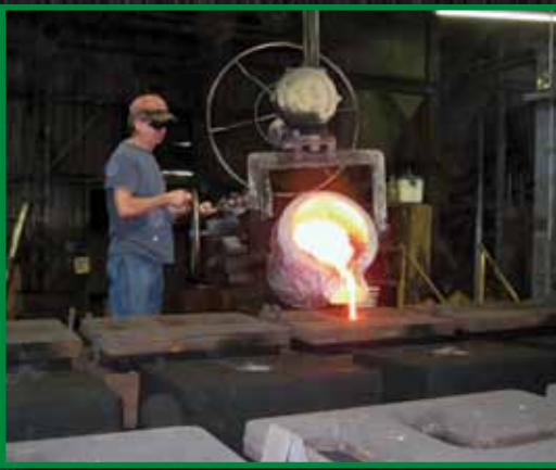
Molten iron is poured into molds produced from the FBO-3 Roberts Sinto.
